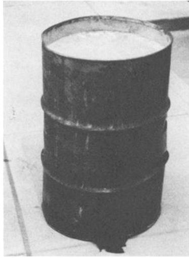
FIG. 1—From Case 1, top view of 55-gal (208-L) drum filled with concrete.
